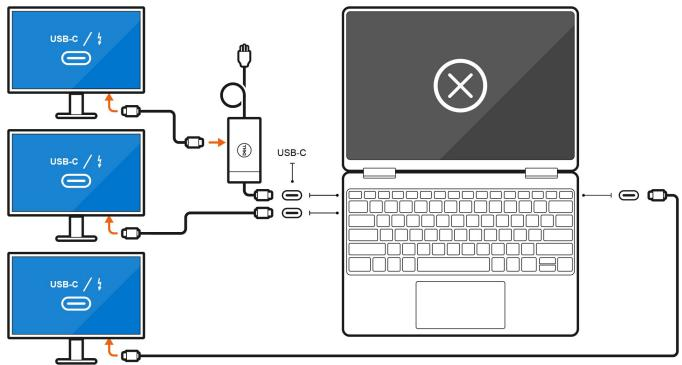
• Connect up to four external displays directly to the WD19TB series docking station and than connecting the docking station to the computer:
