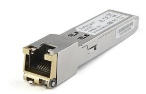
The SFP1GTEMCST is a Dell EMC SFP-1G-T compatible copper transceiver module that has been designed, programmed and tested to work with Dell EMC brand switches and routers. It delivers dependable 1 GbE connectivity over copper cable, for 1000BASE-T compliant networks, with a maximum distance of up to 100 m (328 ft).
