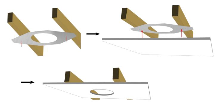
Figure 8. Install bracket and drywall or sheet rock
