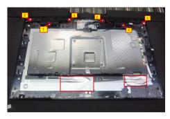
Disconnect the speaker cable away from the board, then release the speakers from the probers of the middle frame. Disconnect the panel lamp cable away from the connectors of the main board and panel.
