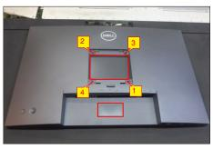
Insert a DP out Cap into the DP out connector. Take a stand base close to the monitor. Fit the two tabs on the upper part of the stand into the grooves, and then lower the stand so that the monitor mounting area snaps onto the stand.
