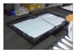
Use a Philips-head screwdriver to lock 11pcs screws
