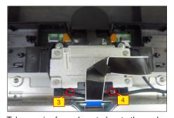
Take a pair of speakers to locate the probers of the middle frame, then locate the speakers' cable to the hooks of the middle bezel, and then connect the speaker's cable to the connector of the main board. Take 1 pcs panel lamp cable to connect the main board with the panel.
