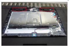
Use a Philips-head screwdriver to remove 4pcs screws for unlocking the camera module with the middle bezel, then disconnect the camera cable from the connector.
