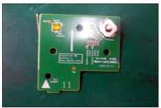
Locate the joystick board to the correct position of the rear cover, then use a Philips-head screwdriver to tighten 3pcs screws for locking the joystick board with rear cover, fix the key cable on the rear cover by 3pcs adhesive tapes on the back of the cable.
