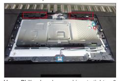
Use a Philips-head screwdriver to tighten 6pcs screws for locking the two speakers with the middle frame, then paste 2pcs aluminum foil on the specific positions to cover the LVDS connector and cables.
