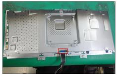
Turn over the bracket and remove the power board and interface board from the bracket chassis module carefully, and then disconnect all of the cables.
