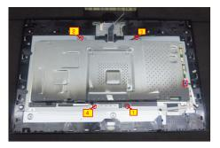
S12 Disconnect the LVDS cable away from the connector of the panel module, then lift up and take away the bracket chassis and put it on a protective cushion.
