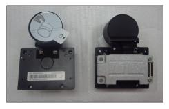
Tear off 2pcs aluminum foil to release the Mic boards
