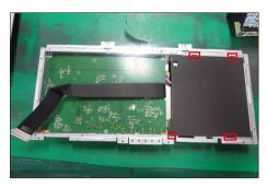
Panel preparation: Take out 1pcs panel module from the carton, remove the protective film by tearing off the tapes, then Examine the panel surface according to inspection criteria. Turn over the panel to place screen faced down for later assembling.
