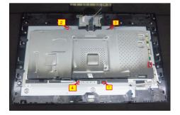
Connect the camera cable to the camera board, then use a Philips-head screwdriver to tighten 4pcs screws for locking the camera unit with the frame.
