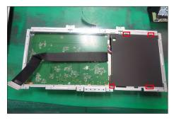
Use a Philips-head screwdriver to remove 7pcs screws for interface board and power board. Turn over the bracket and disconnect the camera cable.
