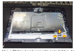
Use a Philips-head screwdriver to tighten 4pcs screws for locking the bracket chassis with the panel, then connect the touch cable to main board.
