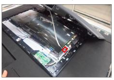
Use a Philips-head screwdriver to remove 3pcs screw for unlocking the joystick board, then tear off all the tapes and release the joystick cable.
