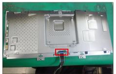
Turn over the bracket chassis, and then take 1pcs black mylar to insert the hooks of the bracket chassis to cover the power board.
