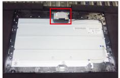
Move the bracket and put it on the back of panel, then connect the LVDS cable to the connector of the panel module.
