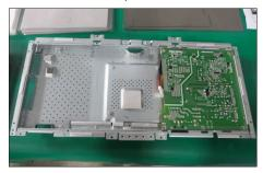
Take a interface board, connect 1pcs LVDS cable to the connector of the interface board, then connect the cable of the power board to the connector of the interface board. Turn over the interface board and locate it into the main chassis. Use a Philips-head screwdriver to tighten 7pcs screws for locking the interface board and power board. Turn over the chassis and connect 1pcs cable to the connector.
