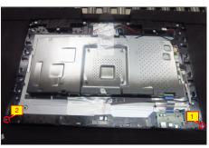
Take 1pcs joystick key, 1pcs joystick board and 1pcs key cable, then assemble the joystick key with board and connect the key cable to the connector of the
