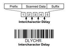
To remove this delay, scan the **Intercharacter Delay** bar code, then set the number of delays to **0**. Scan the **Save** bar code from the **Programming Chart**, beginning on page 227.
