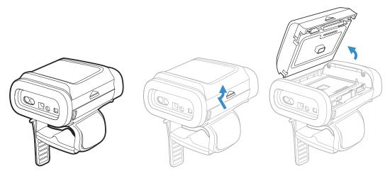
Replace the battery by snapping it in to the 8680i.
