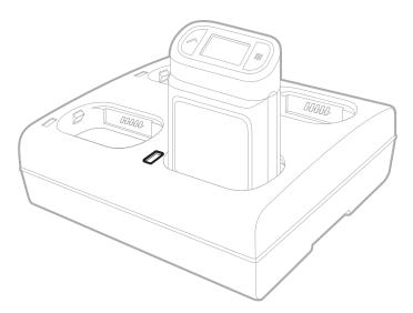
It is important that 8680is are inserted into the charging pocket correctly. Inserting the battery incorrectly could result in damage to the 8680i or the charger.
