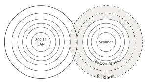
Scan one of the bar codes below to set the 8680i's power output to **Full Power** (100%), **Medium Power** (35%), **Medium Low Power** (5%), or **Low Power** (1%). Default = Full Power.
