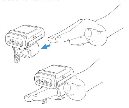
Pull the finger strap to secure it and tuck the excess strap length into the finger guide channel.
