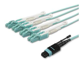
This MPO/MTP to 4x LC breakout cable lets you fan out a single 40Gbps connection from a 40GBase-SR4 QSFP+ transceiver to four 10Gbps LC SFP+ transceivers.
