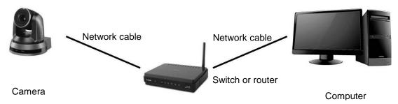
2. To connect directly through network cable, the IP address of the computer should be changed so that it is on the same network segment as the camera e.g.: The factory-preset default IP address of the camera is 192.168.100.100. The computer IP address must be set with the same network segment, such as 192.168.100.101, so that the computer can be connected correctly with the camera
