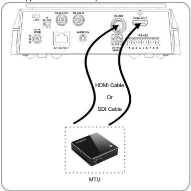
4.3.2 Connecting to an HDTV/computer monitor (HDMI)
