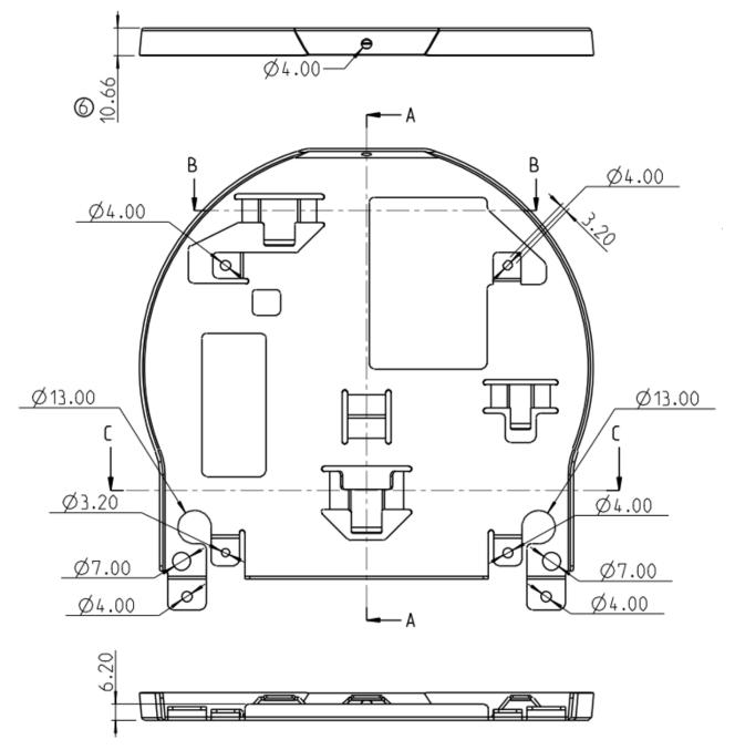
Metal plate A - machine side
