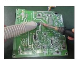
S23-5 Lift the bulk cap. up and away from the PCB.
