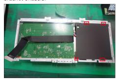
Use a Philips-head screwdriver to remove 7pcs screws for interface board and power board. Turn over the bracket and disconnect the camera cable. (No.1 screw size=M4x8, Torque=7.5 0.5kgfxcm; No.2~7 screw size=M4x8, Torque=7.5±0.5kgfxcm)
