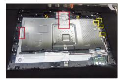
Use a Philips-head screwdriver to remove 1pcs screw for unlocking the USB unit with the middle frame, then disconnect the two USB cables and Mic cable away from the connectors of main board. Release the USB board away from the hook of the middle frame.
