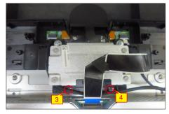
Use a Philips-head screwdriver to remove 4pcs screws for unlocking the bracket chassis with the panel, then disconnect the touch cable away from the connector of the main board.
