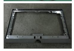
Release the touch key cable away from the panel, S19 then disassemble the front bezel with the panel, then tear off the mylar tape and release the touch board.
