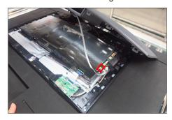
Use a Philips-head screwdriver to remove 3pcs screw for unlocking the joystick board, and then tear off all the tapes on the back of the cable and release the joystick cable from the rear cover.
