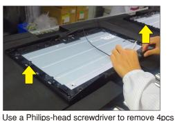
screws for unlocking the left and right Mic boards with the middle frame, then release the two Mic boards away from the middle frame.
