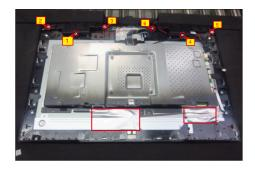
S11 Disconnect the speaker cable away from the board, then release the speakers from the probers of the middle frame. Disconnect the panel lamp cable away from the connectors of the main board and panel.
