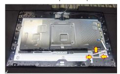
Release the assembled camera unit from the probers of the middle frame and put it aside for later S15 disassembling.
