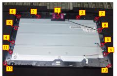
Lift up the middle bezel away from the pane module, S17 then put it on a cushion foam for later disassembling.
