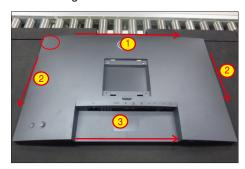
S6 Lift the rear cover up carefully. Disconnect the joystick key cable from the connector of the main board, and then remove the rear cover and put it aside for later disassembling.
