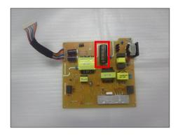
S23-1 Cut the glue between bulk cap. and PCB with a knife.
