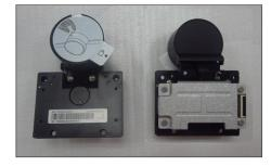
Tear off 2pcs aluminum foil to release the Mic boards Use a Philips-head screwdriver to remove 13pcs screws for unlocking the middle frame with the panel. (No.1~11 screw size=M3x4,Torque=3±0.5kgfxcm; No.12~13 screw size=M2x3.3,Torque=1±0.2kgfxcm)
