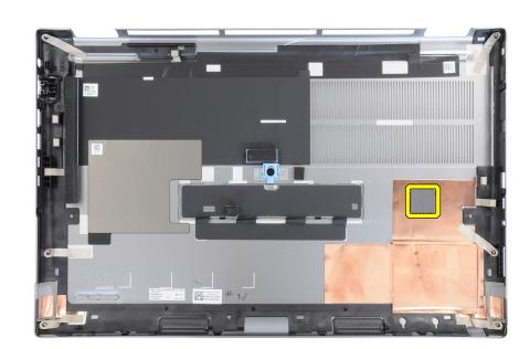
• **Solid-state drive door**: For models shipped with an SSD door, use the latch on the base cover to lock/unlock the door.
