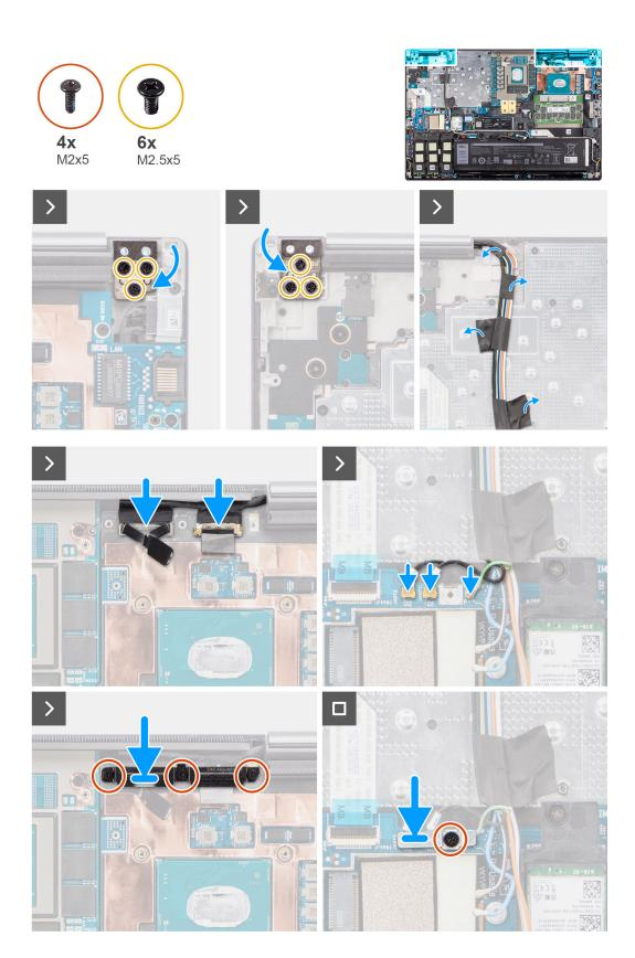
1. (i) **NOTE:** Before installing the display assembly, ensure that the display hinges are opened to a 90-degree angle against the display assembly, to fit the display assembly to the palm rest.
