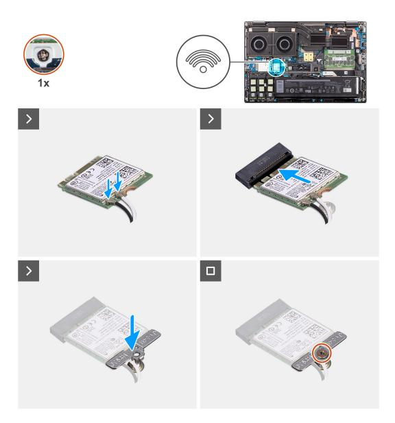
Connect the antenna cables to the WLAN card. The following table provides the antenna-cable color scheme for the WLAN card of your computer.
