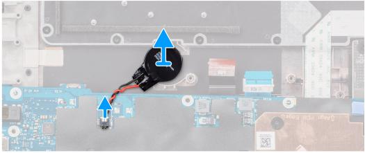
Pry to remove the coin-cell battery, which is located under the system board, from the palmrest while lifting the system board.
