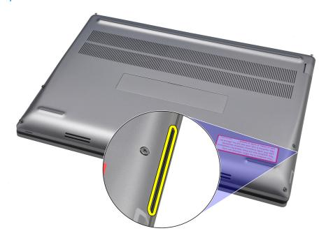
Lift the base cover starting from the bottom edge and push it towards the rear to remove it from the computer.
