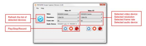
You will then have to use which video device, the resolution and the frame rate to use for the preview/capture. Optional audio source can be selected.
