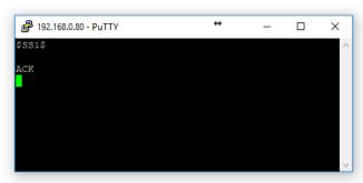
You can use the commands by sending HTTP or TCP requests. For example, you can send an HTTP request by sending it using any browser, for example, to 192.168.0.80:50000/COMMAND. If the command is recognized, you will receive the ACK string.
