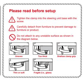
Put the screw through the clamp.
