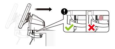
Rotate the screw clockwise while supporting the steering unit and firmly secure.
