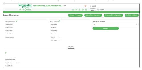
You can perform functions like **Uploading Firmware**, **Uploading Configuration**, **Downloading Configuration** and returning the settings of the Rack PDU to the **Default Settings** from the System Management page. You can also **Restart** the Rack PDU from the System Management page.
