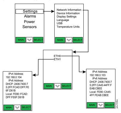
To login to the Web UI, in a standard web browser, enter the IP address you obtained from the Rack PDU:
