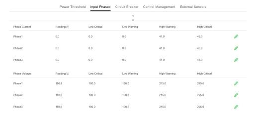
To edit or change the Phase Voltage Settings, click the Edit icon ? to open the **Input Phase Voltage Alarm Setting** dialog boxes. The following settings can be accessed here:
