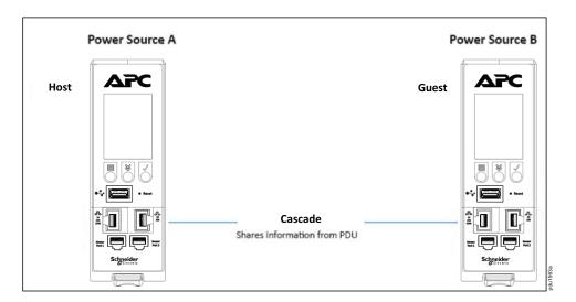
The Redundant Network Access allows secure access of Rack PDU data and statistics on two (2) separate private networks. RNA is used with a redundant power delivery design including two (2) Rack PDUs for each IT rack. The Rack PDUs must be the same SKUs when used in RNA applications.
