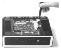
2. Install the SDD bracket to a 2.5-inch SATA SSD with 2 screws.
