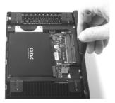
2. Insert an M.2 2242 SSD module into the slot at a 45 degree angle.
