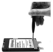
3. Insert the SSD into the socket and gently slide into the connector.
