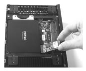
3. Gently press down on the M.2 2242 SSD module, and install the screw.
