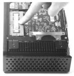
Note: This ZOTAC ZBOX nano accomodates two DDR5 SO-DIMM memory modules. You must install at least one module for the system to function. Windows models include memory pre-installed.
