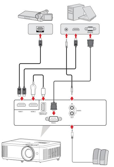
The projector will automatically search for input sources. If multiple sources are connected, press the **Source** button on the projector or remote control to select the desired input.
