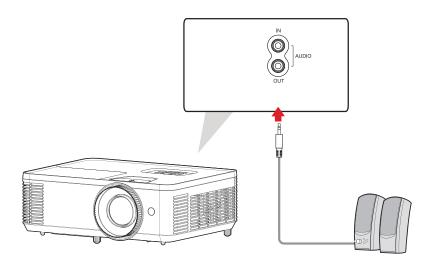
Additionally, you can connect to the **AUDIO IN** port with your device to use the projector's audio output.
