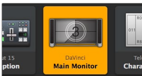
The video destination button will illuminate when selected and displays its current source. In the above example, the destination is the main monitor connected to a DaVinci Resolve suite.
