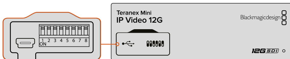
Change settings by adjusting switch 1 with a pen
