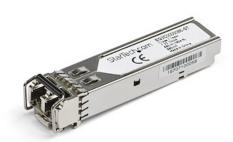
The EG3C0000086-ST is a Citrix EG3C0000086 compatible fiber transceiver module that has been designed, programmed and tested to work with Citrix brand switches and routers. It delivers dependable 1 GbE connectivity over fiber cable, for 1000BASE-SX compliant networks, with a maximum distance of up to 550 m (1804 ft).
