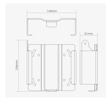
Once the steel plate is mounted to the wall, the Sonos Port simply slides into position and is held securely. A padlock (not supplied) can also be fitted to prevent unwanted removal.
