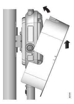
**Step 1** Position and rotate the cover over the AP.
