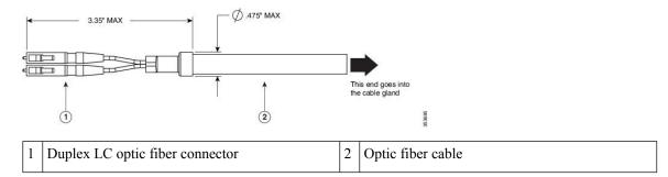
Using caution not to damage the fiber connector end, pass the fiber connector through the adapter gland components. Ensure components are ordered and orientated, as shown in Figure 34: Duplex LC Fiber Optic Cable, on page 40.
