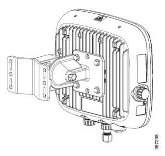
Figure 7: Pivoting Wall Mounting Bracket
