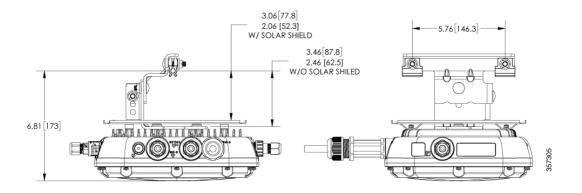
Figure 18: Assembling the cable bracket and Clamps
