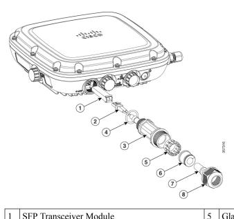
Figure 32: Exploded view of Fiber-Optic cable and Gland assembly
