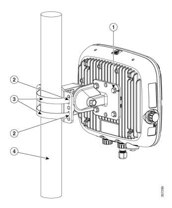
One of four mounting holes for mounting the AP to the bracket
