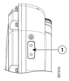
Ground pad, where the ground strap screw holes are located.
