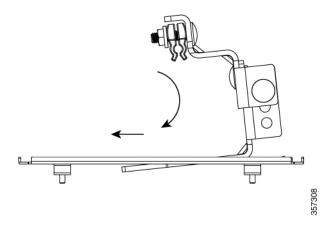
**Note** If needed, reposition the AP on the bracket assembly so it hangs level. Loosen the M8 screws just enough to move on a slotted hole, then re-tighten the screws to 15 lbf-in (17 kgf-cm) of torque.
