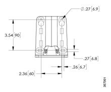
Figure 13: L-bracket AP mount dimensions
