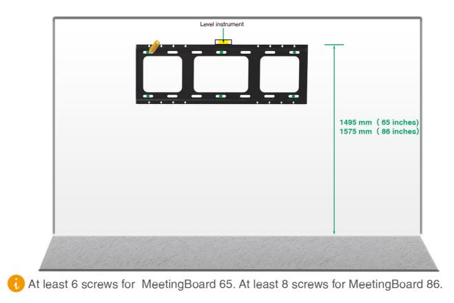
2. Fix the expansion screws/self-tapping screws at the marked positions on the wall
