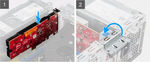
1. (i) NOTE: The Dell Ultra Speed Drive Gen4 card must be installed in the PCIe x4 slot.
