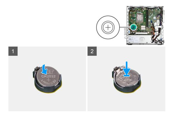
Insert the coin-cell battery into the socket with the positive side (+) label facing up and snap the battery in the socket.
