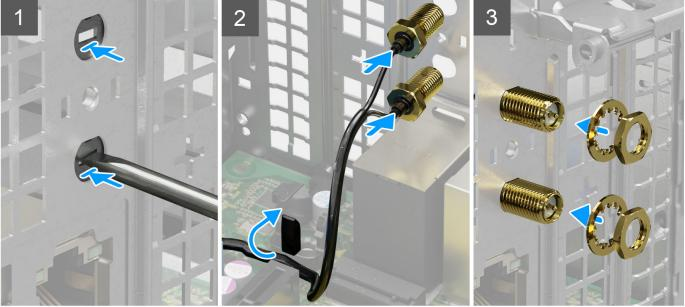
1. Push and remove the antenna cover from the chassis using a screwdriver.
