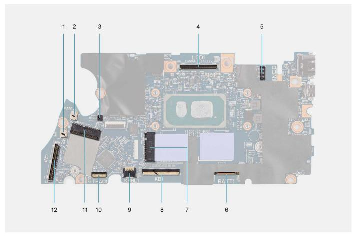
Figure 2. System-board connectors
