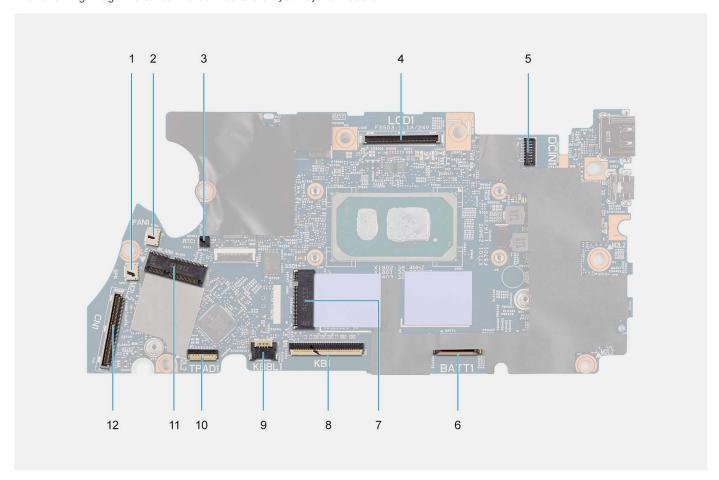
Figure 1. System-board connectors
