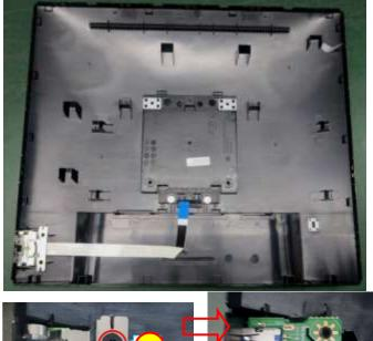
S4.Remove the USB board and key board
