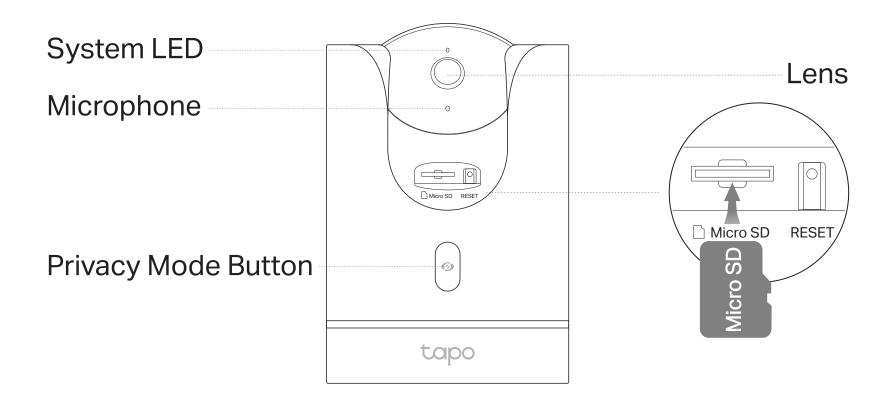
**Note:** Tilt the camera lens up to find the RESET button and the microSD card slot.
