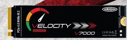
Using the latest Gen 4x4 NVMe controller and 3D TLC NAND, Origin Velocity V7000 offers incredible speeds of up to 7,450/6,750MB/s¹ read/write and up to 953K IOPS³ for exceptional gaming experience. Dominate the competition with rapid file transfers and lightning fast game and application loading times.
