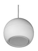
The EN-SPH5T16-W is a compact 5.25" sphere loudspeaker with ABS housing (Ul94 HB) (RAL 9010 equivalent), equipped with a high efficiency full range speaker and a multi tap 100 volt transformer, all certified according EN 54-24.
