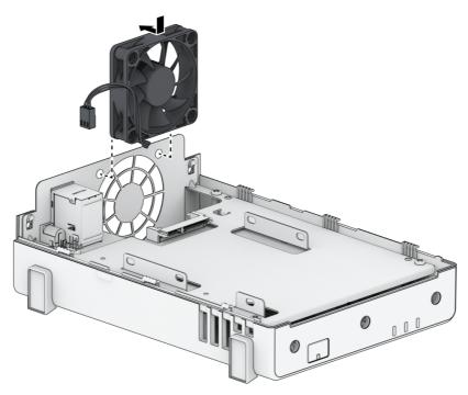
2. Plug the fan connector back in and affix the tape to its original location.
