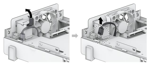
5. Remove the malfunctioning fan.
