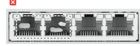
6. Check the interior of the network port for damaged or skewed pins.
