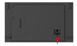
Use a screwdriver to remove 8pcs screws for releasing the handles. (Torque:15±0.5kgf)
