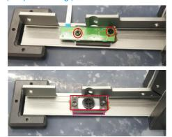
Use a screwdriver to remove 27pcs screws for unlocking the front bezels(top, left, right, bottom). (Torque: 3±0.3kgf)
