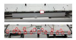
Use a screwdriver to remove 8pcs screws for unlocking the two bracket with the bottom ED holder. (Torque: 3±0.3kgf)
