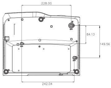
Ceiling mount screws: 3 PCS Screws specs: Φ=4mm L=10mm
