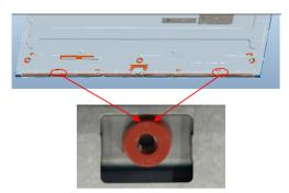
S19 Disassemble mylar from Main SHD
