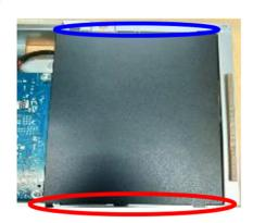
S20 Unlock 8 PCBA screws to disassemble I/F BD, SPS BD from Main SHD
