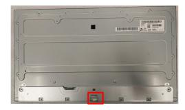
S18 Disassemble 2 plastic BOSS from panel
