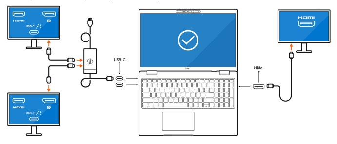
• Connect up to three external displays using direct USB-C or Thunderbolt cables and a direct HDMI cable:
