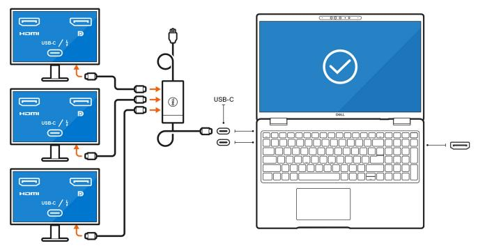
• Connect up to three external displays using a USB-C docking station:
