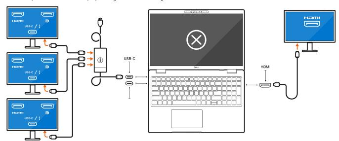
• Connect two external displays using a docking station and two more external displays using a USB-C to HDMI/DisplayPort/ Thunderbolt 4 adapter:
