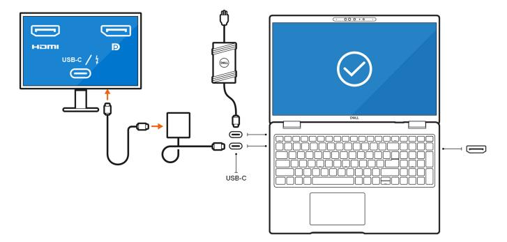
• Connect up to two external displays using a USB-C docking station:
