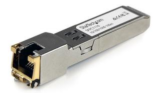
The SFPC1110 is a Cisco SFP-GE-T compatible copper transceiver module that has been designed, programmed and tested to work with Cisco brand switches and routers. It delivers dependable 1GbE (1000 Mbps) connectivity over copper cable, for 1000BASE-T compliant networks, with a maximum distance of up to 100 m (328 ft).
