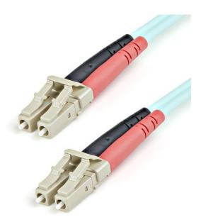
The A50FBLCLC1 1m 850nm Laser-Optimized Multimode Fiber (LOMMF) Aqua Cord features 50/125 micron fiber for high-speed, high bandwidth data transmissions over 10 Gigabit Ethernet and Fiber Channel networks - the perfect solution for fiber cable runs between multiple backbone switches, hubs and routers as well as higher end networking equipment.
