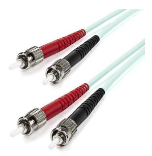
Perfect for fiber cable runs between multiple backbone switches, hubs and routers as well as higher end networking equipment, this high speed 10 Gigabit Multimode Duplex Fiber Cable is terminated with ST connectors on both ends, and is composed of 50/125 micron OM3 aqua fiber to deliver reliable data transfers at blinding speeds.
