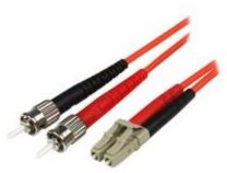
The 50FIBLCST5 5m LSZH LC to ST Fiber Cable features 50/125 micron fiber for high-speed, high bandwidth data transmissions over Gigabit Ethernet and Fiber Channel networks, with support for duplex multimode applications.
