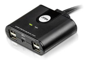
The US224 is a 2-port USB peripheral sharing device that enables 2 computers to share the use of 4 USB devices – a keyboard, mouse and up to two peripheral devices. It eliminates the added expense of having a separate USB keyboard, mouse and peripheral device(s) for each computer. The US224 all-in-one design allows for a neat and tidy installation – no need to connect 2 separate USB cables to the computer, thus eliminating cable clutter.
