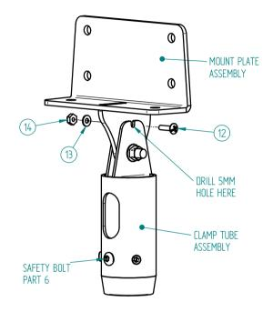
WHEN MOUNTING HEAVY EQUIPMENT AN OPTIONAL LOCKING BOLT (PART 12) MAY BE USED TO SET THE POLE VERTICAL AT ANY CEILING PITCH UP TO 45°.
