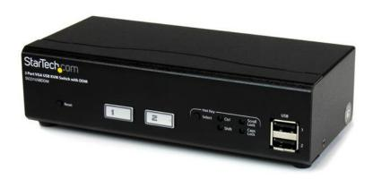
The SV231USBDDM 2-Port USB VGA KVM Switch lets you control 2 VGA, USB-equipped PCs using a single peripheral set at high-definition VGA resolutions up to 1920x1440.
