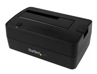
Unleash the power of USB 3.1 Gen 2 (10 Gbps) with this single-drive docking station. It supports both 2.5" and 3.5" form factors for solid-state and hard drives, with a high drive capacity of 6TB.
