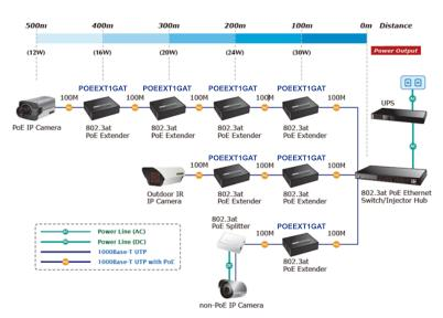
Each PoE Extender unit requires ~3.2 Watts maximum to power the unit itself. Check the total power consumption of your devices and the PoE Extender units before setting up in a daisy chain configuration. If the overall power consumption is overloaded, the local PSE could shut-down the entire power system. Each cable segment is limited in 100m using standard RJ45 terminated CAT5 or higher Ethernet cable. Any other non-standard cable or distances above 100m could result in unstable connections.
