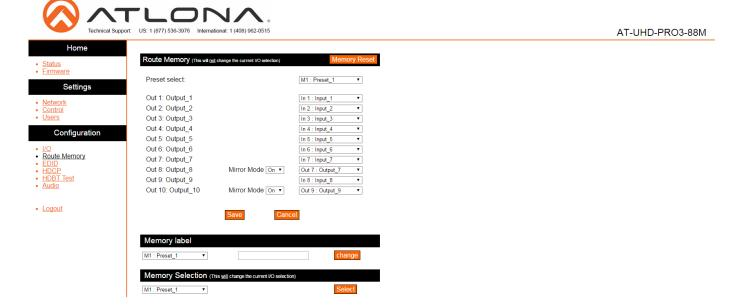
The Route Memory page provides set up, labeling, and configuration of multiple preset memories for fast and easy control.
