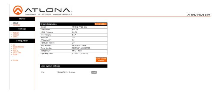
The home page will allow the user to see the general system information, download the matrix log, and save/load system settings. The information displayed will help figure out if the matrix is up to date, how long it has been running, and other key information.
