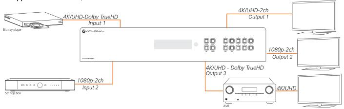
On default, all devices in the diagram will work at 1080p. If a device is not syncing or a different resolution is required, internal EDID or EDID copy and load should resolve these issues. The UHD-PRO3 can copy and store up to 10 EDIDs to memory.
