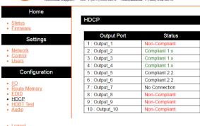
The HDCP page provides a quick way to see whether a display is HDCP compliant or not and the version supported. This page will give multiple status readouts: No Connection, Compliant 1.X, Compliant 2.X, and Non-Compliant.
