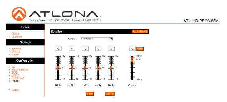
The audio page supports adjustment of 5 band EQ for the analog audio outputs ensuring the best audio performance for each zone. 5 band frequency options at 63Hz, 250Hz, 1kHz, 4kHz, and 8kHz as well as zone output volume and mute.
