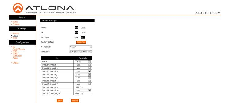
The control page will allow simple functions to be changed. Turn the matrix on/off, IR front panel receiver window on/off, and front panel key lock on/off. The time zone and baud rates (for matrix and zone outputs) can be altered as well.
