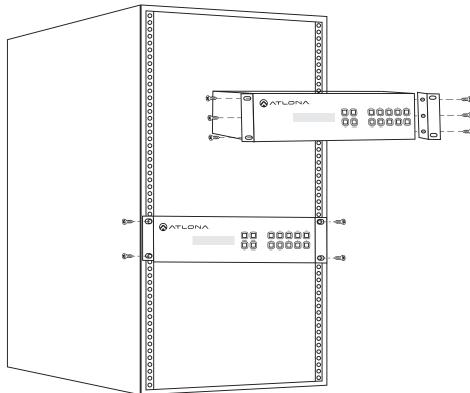
To rack mount the UHD-PRO3-88M unit: use the rack mount ears, the 6 screws from the sides of the UHD-PRO3-88M, and 4 rack screws.
