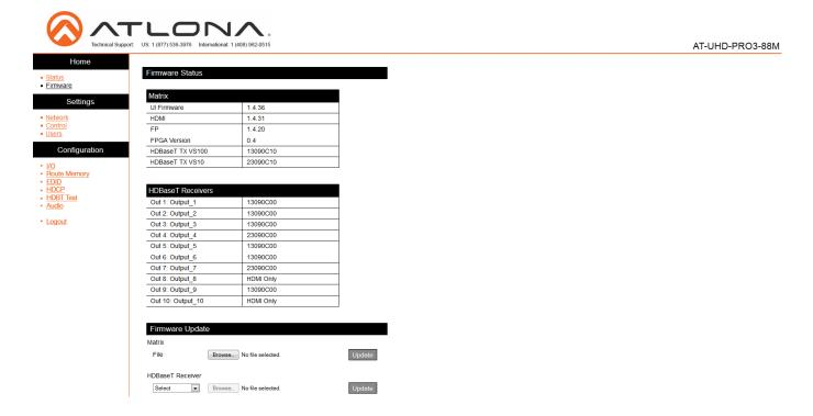
The firmware page displays the matrix, HDBaseT transmitter chips, and HDBaseT receivers firmware version and provides an easy way to update.
