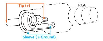
**Note:** Pin outs may vary, please refer to the audio device's manual to ensure a correct connection. **Important!** When terminating cables, please ensure exposed adjacent wires do not touch. This may result in a short that can damage connected devices.
