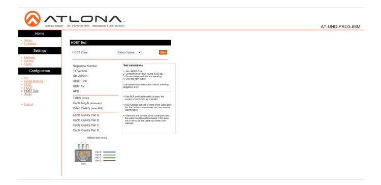
The HDBT page provides testing of Ethernet cables connected to the HDBaseT port on the matrix. To perform an HDBaseT test, do the following:
