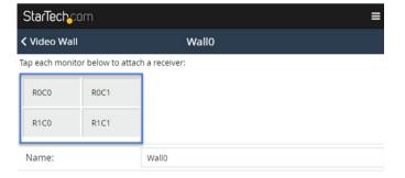
You'll need to use this example to specify which receivers are represented within your video wall configuration. Select the receiver from the video wall example to display a list of all connected receivers, then choose the receiver that corresponds with the proper location within your video wall configuration.
