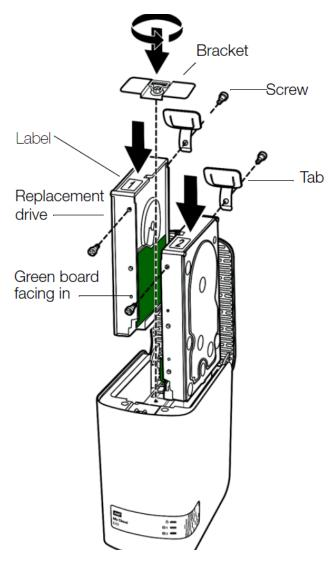
Note: You'll need a phillips-head screwdriver for this procedure. Also, the power and network cables are not connected when you do this.
