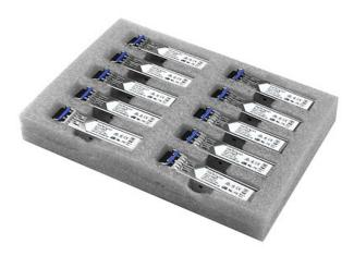
The GLCLHSM10PST is a Cisco GLC-LH-SM compatible fiber transceiver module that has been designed, programmed and tested to work with Cisco brand switches and routers. It delivers dependable 1 GbE connectivity over fiber cable, for 1000BASE-LX/LH compliant networks, with a maximum distance of up to 10 km (6.2 mi).
