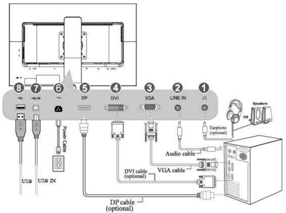
Figure.2. Connecting to a PC
