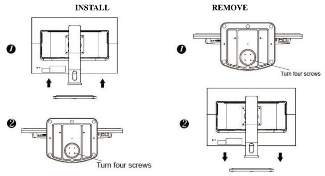
Figure.1. Installing and Removing the Base
