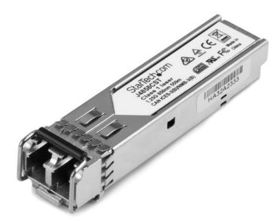
The J4858CST is an HP J4858C compatible fiber transceiver module that has been designed, programmed and tested to work with HP® brand switches and routers. It delivers dependable 1 GbE connectivity over fiber cable, for 1000BASE-SX compliant networks, with a maximum distance of up to 550 m (1804 ft).
