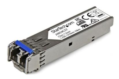
The J4859CST is an HP J4859C compatible fiber transceiver module that has been designed, programmed and tested to work with HP® brand switches and routers. It delivers dependable 1 GbE connectivity over fiber cable, for 1000BASE-LX compliant networks, with a maximum distance of up to 10 km (6.2 mi).
