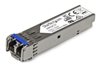
The J4859CST is an HPE J4859C compatible fiber transceiver module that has been designed, programmed and tested to work with HPE brand switches and routers. It delivers dependable 1 GbE connectivity over fiber cable, for 1000BASE-LX compliant networks, with a maximum distance of up to 10 km (6.2 mi).
