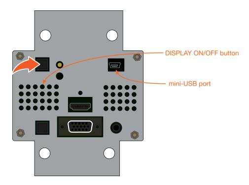
After a few seconds, a folder with the name USB UPDATER, will be displayed. Release the DISPLAY ON/OFF button.
