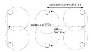
**STEP 5** Using your sketch of the room, create a Bass Loudspeaker Layout with the correct number of bass modules to meet your Coverage Requirement.
