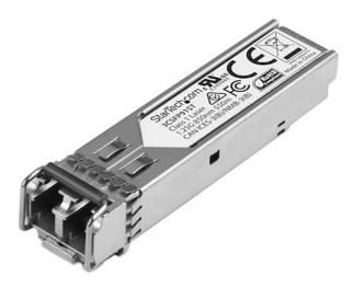
The 3CSFP91ST is an HPE 3CSFP91 compatible fiber transceiver module that has been designed, programmed and tested to work with HPE brand switches and routers. It delivers dependable 1 GbE connectivity over fiber cable, for 1000BASE-SX compliant networks, with a maximum distance of up to 550 m (1804 ft).
